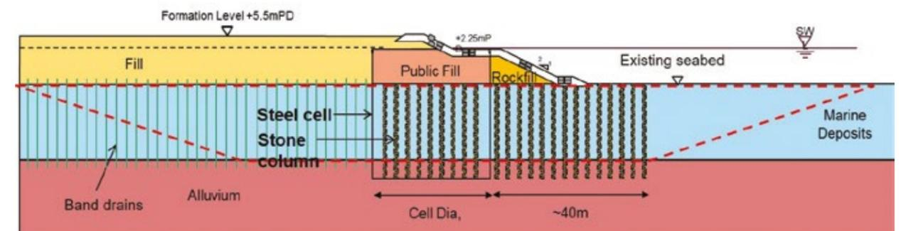
Non-dredged method: stone columns are installed to provide support for filling materials above and serve as porous drains, allowing the marine sediment to be left in place.
