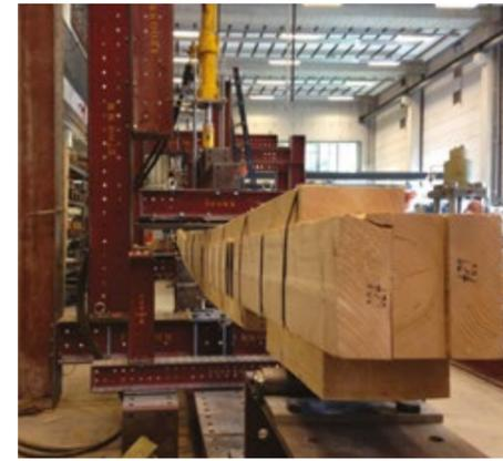
Lab tests for the composite beams
