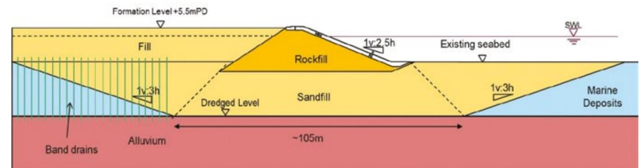
Conventional dredged method: marine sediment is dredged away and disposed of, then backfilled with a similar volume of sandfill/rockfill.
