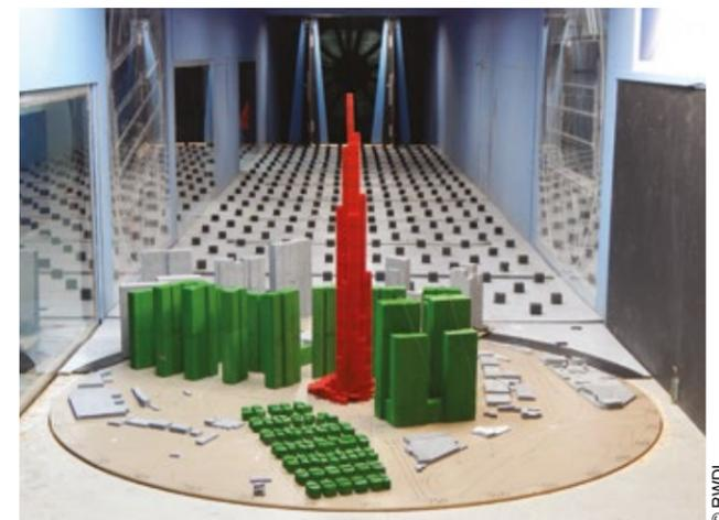
■ Wind tunnel test for Landmark 81
