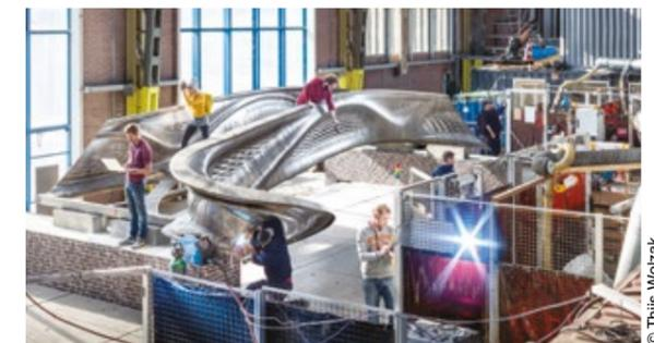
This robot-printed pedestrian bridge in Amsterdam, which welds traditional steelwork and advanced digital modelling, is an important marker for the future of architecture and construction. Arup is the project's lead engineer.
