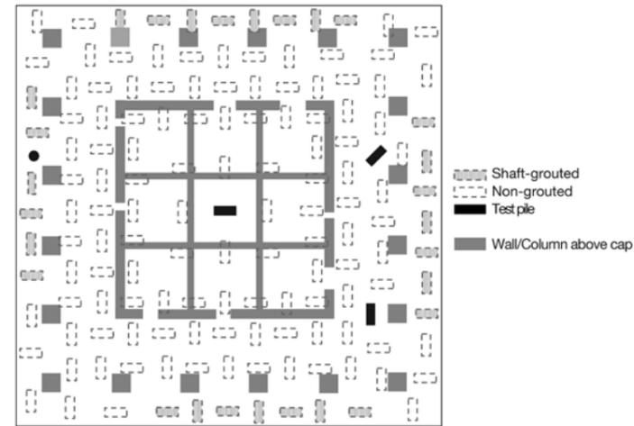
Final pile layout showing the barrette piles orientated to suit the specific loading requirements of each location
