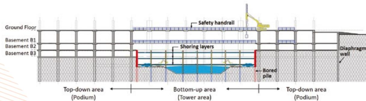
Basement construction showing top-down and bottom-up zones: (top) plan view, (bottom) side view
